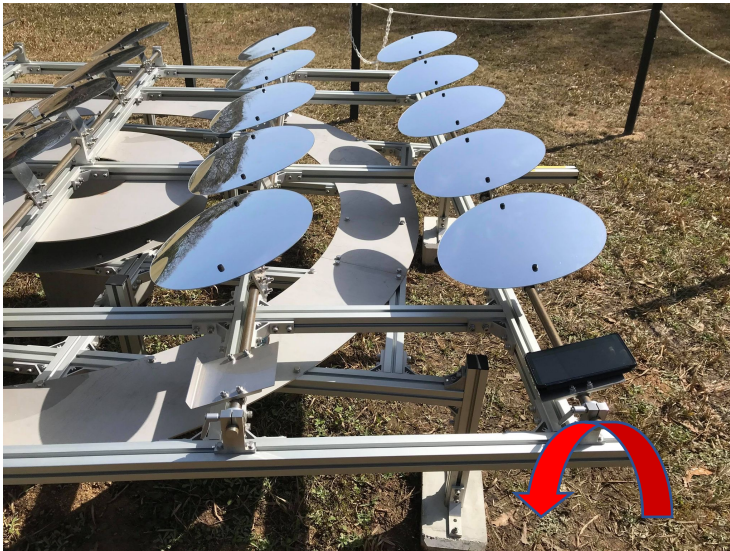
A key for tilt angle adjustment
