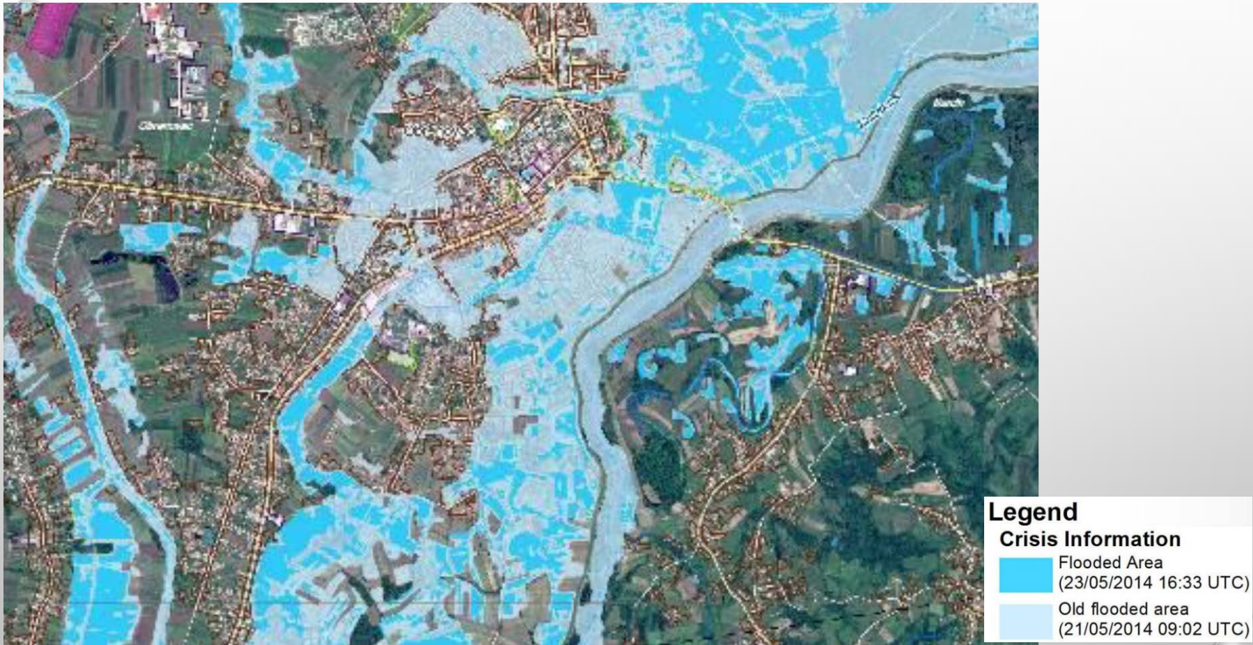
Figure 6: It is suggested to adopt filled polygons without outlines if the flood layers can be derived with a high level of reliability. For example light blue can show the “older” information while darker blue shows the newer information layer. Transparency may allow better interpretation due to better readability of the layer context.
