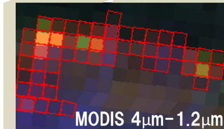
MODIS 4 \mu m-1.2 \mu m We can detect wildfire as red rectangle pixels, however, we do not know exact place.
