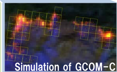
Simulation of GCOM-C Small pixel (250m) and 2.2 \mu m SW allow us to find exact place of wildfire.
