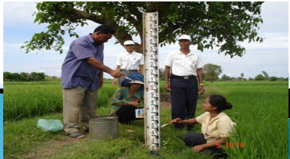
Water level pole built in at the rice field
