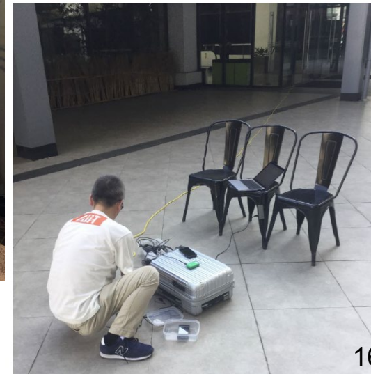
Receiving QZSS signal through receiver
