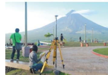
Fieldwork at Mayon to collect ground control points for DEM validation in Feb. 2010
