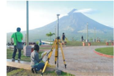
Fieldwork at Mayon to collect ground control points for DEM validation in Feb. 2010
